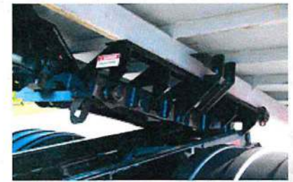
Rear container transition supports w/ pass through rear hold downs
