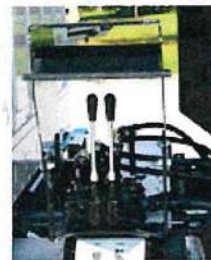
Secondary outside manual control valve
