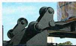
Dual rear rollers are ductile cast iron 6" OD and flared sides w/ bronze bushing
