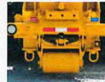
Rear hydraulic stabilizer with 10" ground roller
