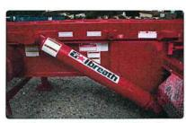
2 cylinders are mounted on the outside of the rails to provide stability when loading heavy boxes.
