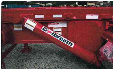
2 cylinders are mounted on the outside of the rails to provide stability when loading/unloading heavy boxes.
