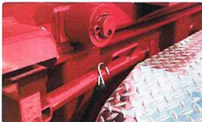
All trailer hoists have dual safety props to add extra security when the hoist is in the up position. 7 rollers per side help aid the container as it is loaded or unloaded on the hoist. Each roller is equipped with a bearing and a grease fitting for easy rolling and maintenance.
