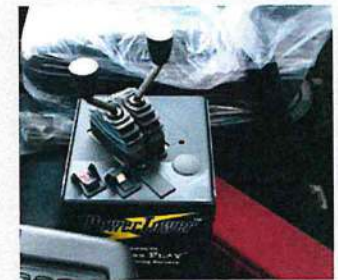
Inside air controls center mounted in ergonomic Power Tower featuring Plug And Play™ wiring
