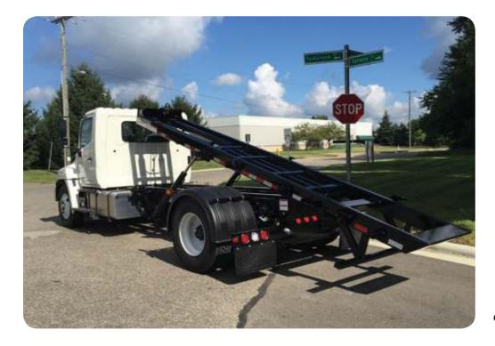
Part No: H20-OR-140 20,000 lb Truckhoist 140" Cab Axle 19' Rail • Up To 16' Box Recommended Container Length 16' 10, 15, 20 yd (with Tarp Space 152"-154")
