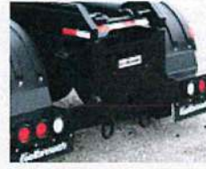
Rear apron & bumper assembly complete w/ LED lighting & pintle/reese adaptable
