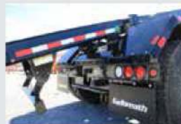
Heavy-duty rear apron w/ split bumpers & recessed LED lighting
