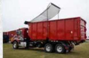
U5-OR-174 shown with Pioneer® tarp, front and rear ratchet hold downs, lift axle, and poly tri-axle fender options
