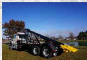
U5-OR-174 shown with Pioneer® tarp, LED safety lighting, Hi-Vis yellow tail, rear ratchet hold downs, rear window screen, fire extinguisher, and poly tandem axle fender options
