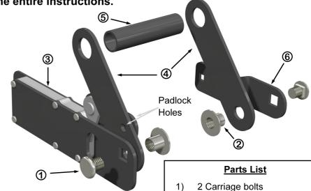
The Lock Release™ Kit CL comes preassembled (Pipe not included). However, if parts need to be replaced, they can be purchased separately. Channel lock pliers will be needed to remove the flange nuts and disassemble the kit.
