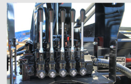
Inside air controls in power tower or integrated into center console on cab over trucks; Secondary outside manual controls at main control valve
