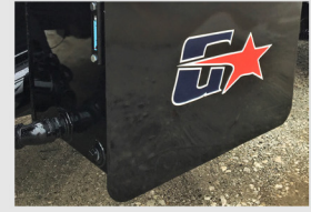
Steel hydraulic tank side mounted with 3 micron filtration, dual sight/temp. gauge & air breather
